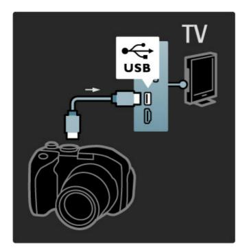
If the list with the content of the camera does not appear automatically, your camera might need to be set to transfer its content with PTP (Picture Transfer Protocol). Read the user manual of the digital photo camera.
